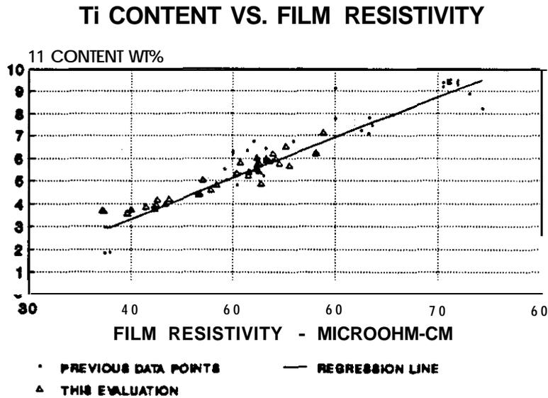
Figure 2. With W-Ti conical style targets, Ti content in the films decreases through life from 7 to 3.5 at%
