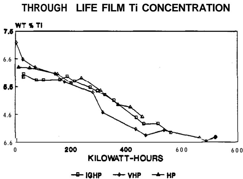
Figure 3. With the decrease in film Ti content, there is a corresponding decrease in the bulk film resistivity. When a full erosion zone RMX™ style target is employed, the fall-off in film resistivity is minimized.
