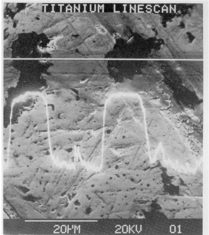
Figure 2- Concentration profiles in the W/Ti alloy.
